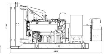
Drawing above for illustration purposes only, based an standard open power 400 Volt engine-generator set. Lengths may vary with other voltages. Do not use for installation design. See website for unit specific template drawings.
