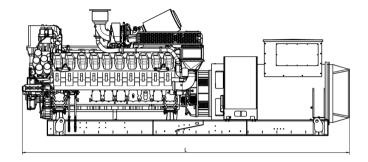
Drawing above for illustration purposes only, based an standard open power 11 kV engine-generator set. Lengths may vary with other voltages. Do not use for installation design. See website for unit specific template drawings.
